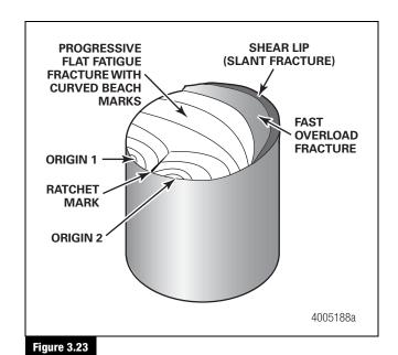
Reverse Bending Fatigue (Fatigue Fracture)
