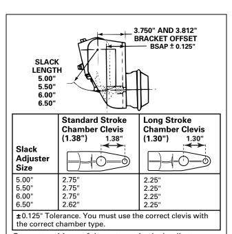
Correct positions of the automatic slack adjuster are 3.750-inch and 3.812-inch offsets only. For other bracket offsets, refer to the vehicle manufacturer's specifications.
