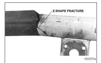
This axle failed in a bending fatigue mode that began at a weld location. The beach marks start at the initial fatigue point and move away from it.
