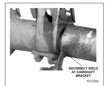
The camshaft bracket incorrectly welded on this trailer axle created a stress riser, which caused the axle to fail.
