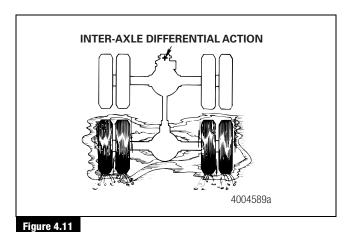
In axles without an oil pump, centrifugal force displaces all of the oil between the cross and pinions, and heat created by friction causes these parts to seize. Sometimes differential pinions become so hot, they weld to the mating surfaces of the differential assembly.
