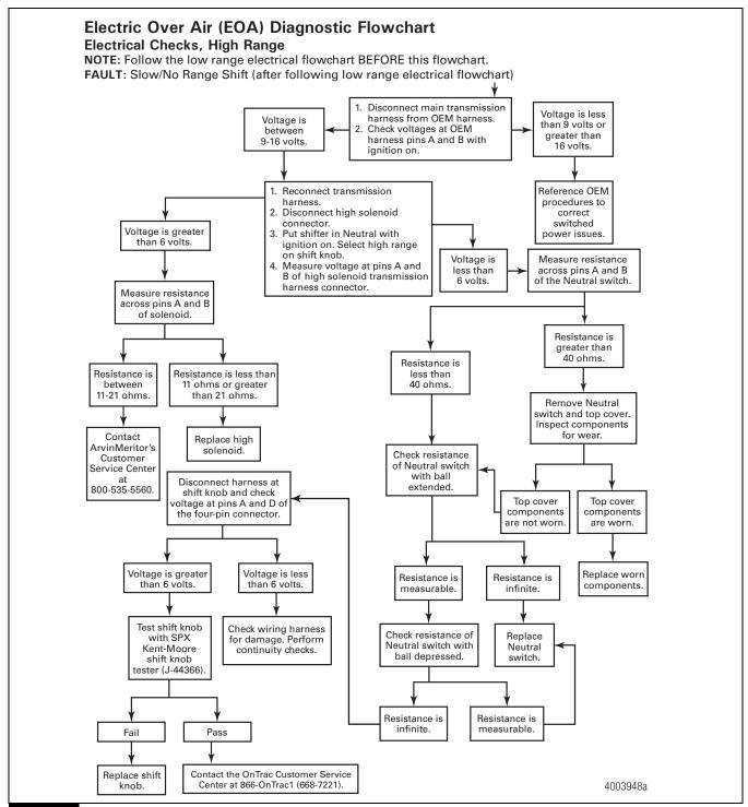
When you find the fault, follow the recommended service procedures to repair it and then test the system. If a fault still exists, or if you find a new one, repeat Steps 1-3 above until you've repaired all the faults.
