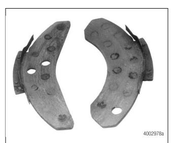
Excessive wear removed the linings from these disc brake pads and caused metal-to-metal contact with the rotor. The result was not only new pads, but a new rotor as well.
