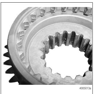
**CLUTCHING TEETH DAMAGE DUE TO TORSIONAL VIBRATION**
