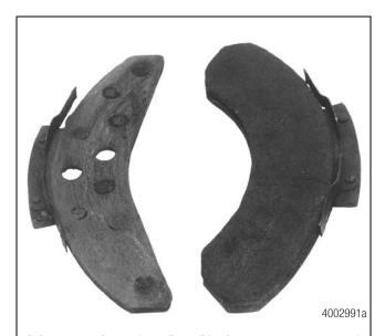
Paint or corrosion on the caliper slide pins can cause uneven pad wear and reduced braking ability. These pads show the results of a corroded slide pin, as well as a failure to check the brakes periodically.
