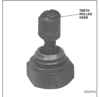
The teeth on this pawl are stripped, metal rolled over the top from turning the slack adjuster nut in the incorrect direction. Simply remove the pawl before manually adjusting or backing off the slack adjuster. Be sure to reinstall the pawl after adjustment.
