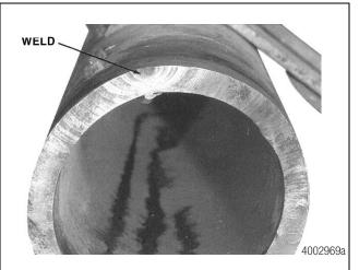
This axle failed in a bending fatigue mode that began at a weld location. The beach marks start at the initial fatigue point and move away from it.
